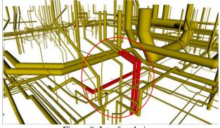
Figure 9: Interfered pipes
