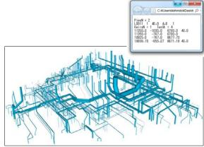
Figure 3: 3-D display of all pipes and data of a pipe
